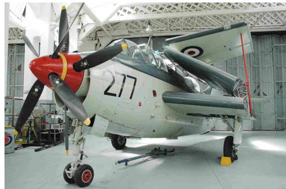
The Fleet Air Arm's Fairey AS6 Gannet anti-submarine plane not only had the unusual double fold by also sported an Armstrong-Siddeley double Mamba engine. Two Mambas were mounted side by side and spun counter-rotating propellers. The aircraft could be flown on one of the engines, saving fuel and increasing endurance.
