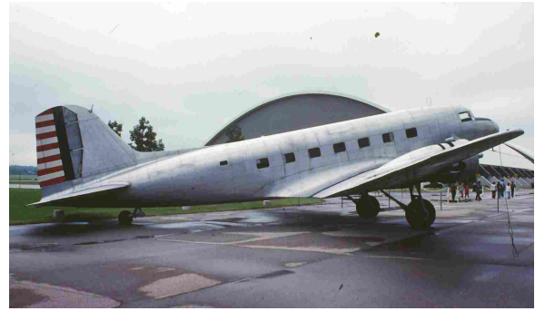
USAAC C-39 at the Museum of the USAF The C-39 is a hybrid of DC-2, DC-3, and B-18 parts.
