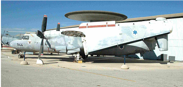
An Israeli Air Force Grumman E-2C Hawkeye at Hatzerim conserves space by rotating the wings and folding the parallel to the fuselage. In Israeli service the aircraft is known as the “Daya” which means kite.
